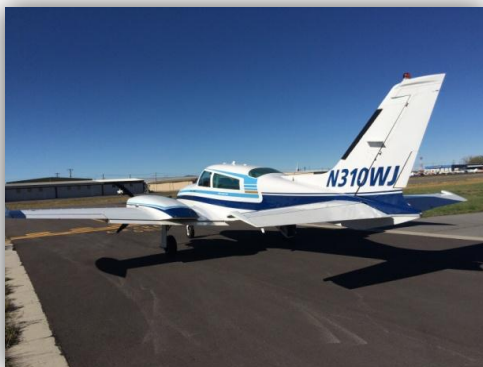
Exhibit 3: The imagery acquisition platform for the Teton County project was a Cessna T310. Our 310 has been customized for imagery and other airborne sensors with an upgraded power system and avionics. The stability of the Aztec is ideal for imagery collection
