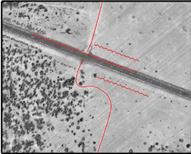
Features Traced on LiDAR Intensity Image Scale 1:1000
